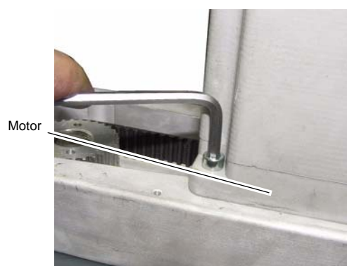
Fig.4-36: Screw the motor
