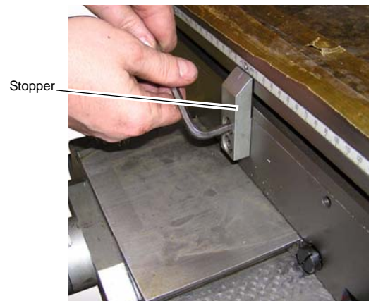
Fig.6-10: Disassemble stopper
