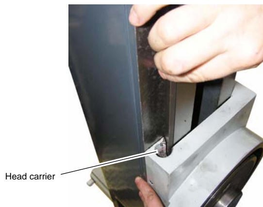
Fig.6-37: Mount the housing
