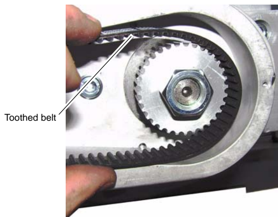
Fig.4-8: Attach the toothed belt
