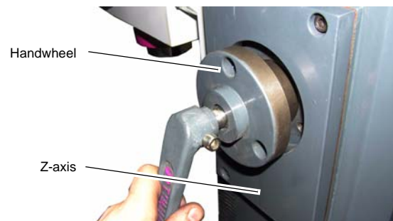
Fig. 4-38: Remove the handwheel
