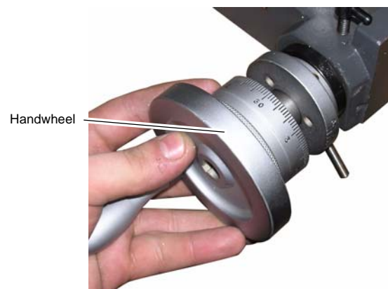
Illustr.4-2: Pull off handwheel
