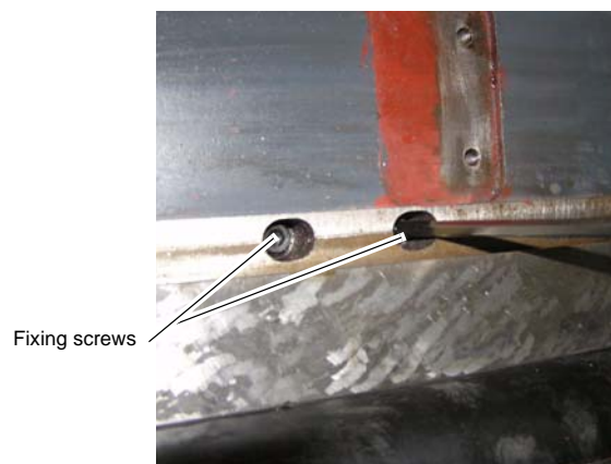
Fig.6-24: Turn in the screws
