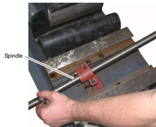
Fig.6-15: Remove the spindle
