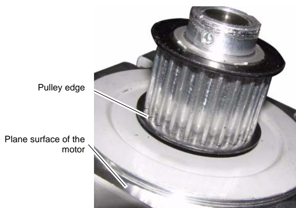
Fig.4-9: Mount the pulley of the motor
