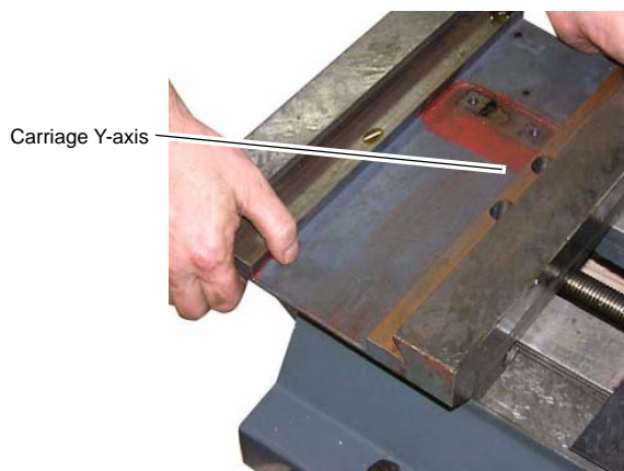
Fig.6-17: Take off the carriage
