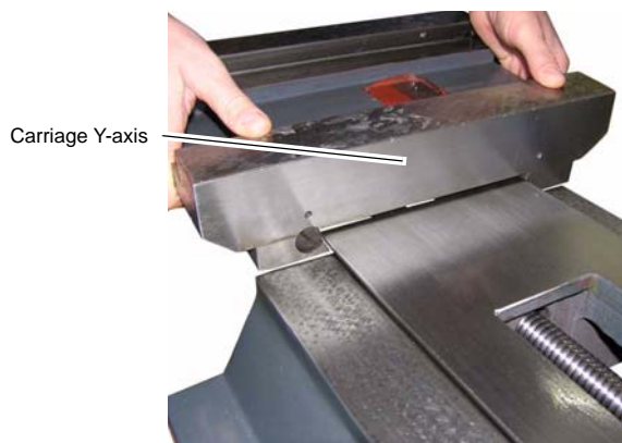
Fig.6-23: Assemble the carriage
