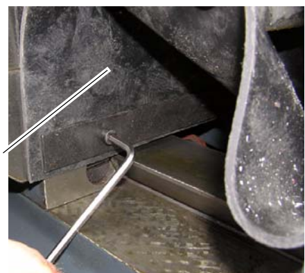
Fig.6-9: Disassemble the rubber cover
