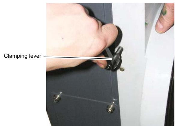
Fig.6-3: Unscrew the clamping lever
