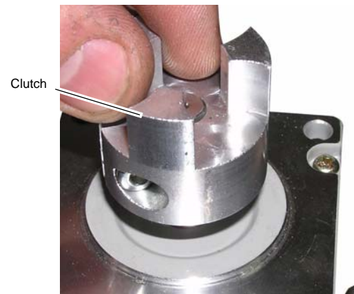
Illustr.4-8: Clutch on the motor
