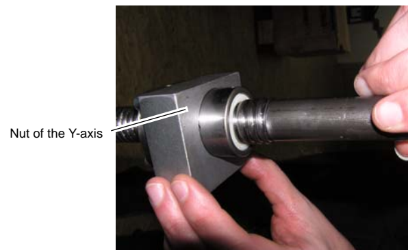
Fig.6-20: Disassemble the nut
