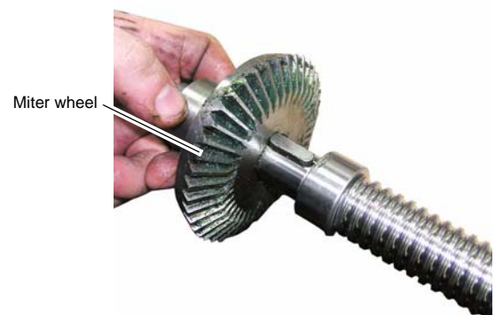
Fig.6-34: Mount the miter wheel
