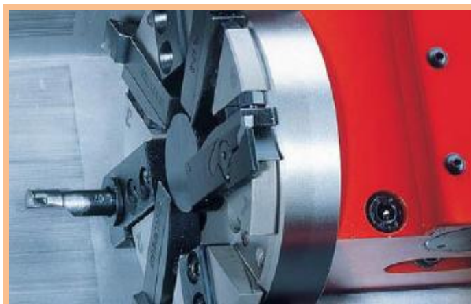
Obr. 6.9 Revolverová hlava CNC soustruhu CONCEPT TURN 105 [17]
