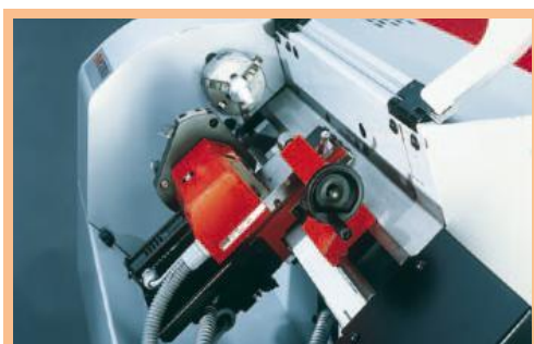
Obr. 6.6 a 6.7 Revolverová hlava CNC soustruhu CONCEPT TURN 55 [17]
